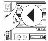
1. Press the back arrow to return to the Audio Routing screen
