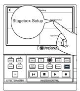
3. Press the Stagebox Setup button on the screen.
