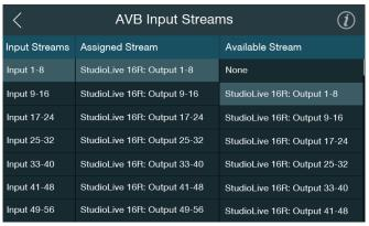
The Input Stream list and the Available Stream list can be scrolled by touching the list header or any where in the list and turning the encoder under the screen. Inputs 57-64 do not show until you scroll down. To change a routing, press the Input Stream to which you'd like to route and then use the value encoder to scroll through the Available Streams list on the right. Tap on the desired routing to patch it.
