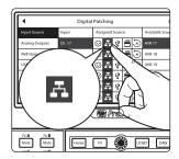
3. Select Input Source and scroll to the desired channels. Assign each to the Network source by pressing the Network button next to each Input.
