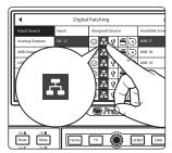
3. Select Input Source and scroll to the desired inputs. Assign each to the Network source by pressing the Network button next to each Input. To assign multiple Network sources at once, press and hold the Network button until the Select buttons flash, then press the Select button for every channel for which a Network source should be engaged. This will patch the Network source on each channel you select.
