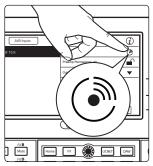
**Power User Tip:** In applications where you are using multiple NSB-series stage boxes of the same model, you can press the Identify button. This will flash Power / Network LED on the top panel red and green on the currently selected NSB, allowing you to quickly locate your selection.
