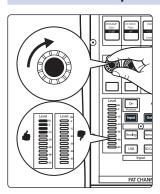
Once the Network input has been selected on the StudioLive Series III console mixer, you can remote control the preamp level and phantom power for your rackmount mixer from the top panel of your console mixer.
