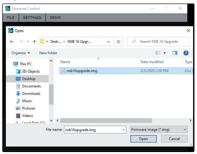
5. Once the file is accepted, the update process will start automatically. This process usually takes 1-2 minutes. After completing, the unit will reboot.
