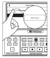
To edit the default AVB Routing between your two mixers, press the AVB Inputs button on the Touchscreen.
