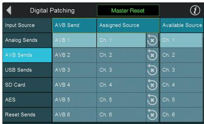
Using the same example above, if you change the Assigned Source for AVB1 to Channel 3 in the Available Source list, and then assign AVB Input Streams 1-8 to Inputs 1-8 on the receiving console, Channel 1 on the receiving console will get its network source from Channel 3 on the transmitting console.
