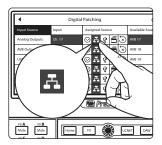
Select Input Source and scroll to the desired channels. Assign each to the Network source by pressing the Network button next to each Input.
