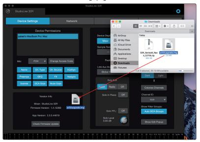
UC Surface will immediately send the firmware update file to the mixer and it will begin the firmware update. A progress bar will be displayed in UC Surface showing the firmware update transfer to the mixer.
