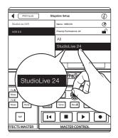
The preamps on NSB-series stage boxes can be controlled from any StudioLive Series III mixer on the network. When you have a stage box feeding more than one mixer, it is recommended that you give only one mixer permission to adjust the NSB preamp levels. In our example, we will be giving permission to the StudioLive 24 at Front-of-House.
