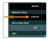
3. The Network clock should be set to Internal.
