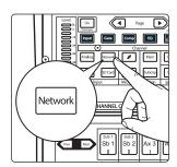
**Power User Tip:** The Network Source can also be enabled for each channel individually from the Fat Channel. Using the Digital Patching screen allows you to assign the sources to multiple channels at once.
