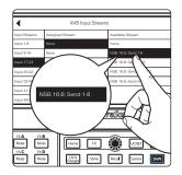
3. Select desired NSB AVB Sends from the Available Stream list to patch the corresponding physical NSB inputs to the desired channesl on your mixer.
