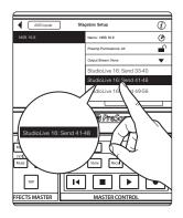
6. Select the AVB Output Sends you'd like returned to the physical outputs on your NSB stage box. Because the AVB streams must be routed in banks of 8, you can only source these outputs from one mixer on the network.
