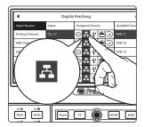
3. Scroll to Inputs 9-32 and assign each to the Network source by pressing the Network button next to each Input.
