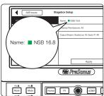
**Power User Tip:** Once send streams from your mixer have been successfully patched, you will see a green status indicator next to your NSB stage box in the setup screen. The light on the front of the NSB will also turn blue, indicating that clock is synced between the mixer and the NSB.
