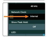
3. The Network clock should be set to Internal.
