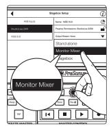
After completing the steps in *Section 4.2*, select Monitor Mixer Mode for your rack mixer from the Stagebox Setup screen on your StudioLive console mixer.
