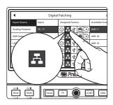
3. Select Input Source and scroll to Inputs 17-32. Assign each to the Network source by pressing the Network button next to each Input.
