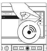
**Power User Tip:** In applications where you are using multiple NSB-series stage boxes of the same model, you can press the Identify button. This will flash the Power Network LED on the front of the selected NSB stage box from green to red, allowing you to quickly locate your selection. You can also rename the NSBs from this screen by touching the NSB name to the immediate left of the Identify button.
