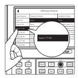
2. Select the desired bank of AVB inputs on your mixer from the Input Streams list.
